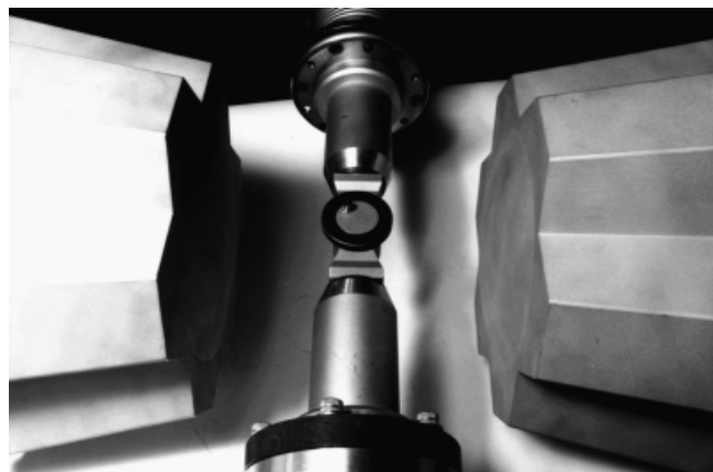
Fig. 1. The spectrometer used for the ^{208}\text{Pb}(^3\text{He}, d^*\gamma\gamma)^{209}\text{Bi} -experiment. One can see the germanium front-ends of the two CLUSTER detectors at a distance of 8 cm from the target which resides in a small chamber.
